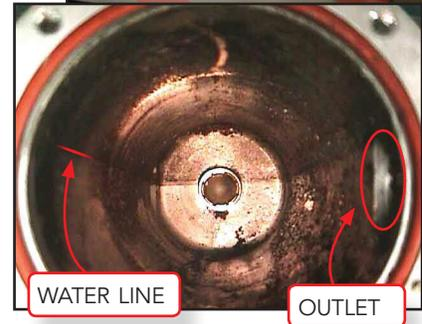
*This heater was mounted with the outlet facing sideways. The coolant never reached the top portion of the tank. This exposed the elements to air and eliminated the heater's ability to "pull" cold coolant from the engine. It is critical that the heater is completely full of coolant at all times. This means the outlet of the heater must be at the highest point of the heater for it to work correctly.*
