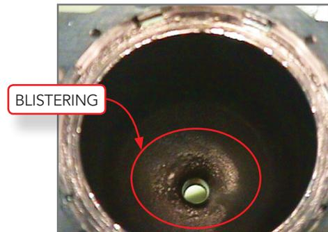
*Blistering on the inside of a thermosiphon heating tank is a tell-tale sign of a flow restriction problem. If coolant is unable to circulate properly, it may overheat in the tank, eventually causing heater element failure.*
