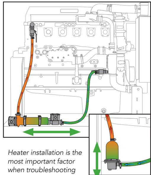
*Heater installation is the most important factor when troubleshooting a thermosiphon heater.*
