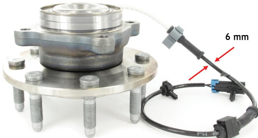
*The 'Classic' Style (GMT 800) has a passive ABS system and a thicker ABS cord than the new style (GMT 900).*
