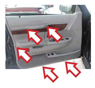
**STEP 2:** Use panel retainer remover to carefully pry-up the master switch assembly.
