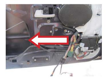
**STEP 15:** Remove the three (3) screws attaching the window lift motor to the window regulator.
