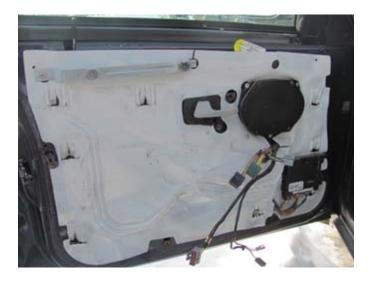
**STEP 6:** Install the water shield.
