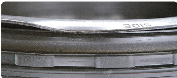
**Dented, scarred sleeve assembly:** This may be caused by improper installation preparations such as not lubricating the I.D. and O.D. of the seal, a poorly prepared hub, or the use of hard-faced tools or seal driver. **Remember:** the Scotseal PlusXL is hand installable. No tools are required.
