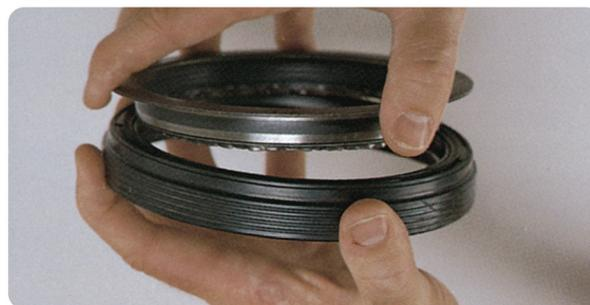
Carefully separate the two components. Then set the seal component aside and carefully review the sleeve component.
