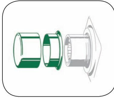
Place SKF SPEEDI-SLEEVE on to the shaft and then place special installation tool over the sleeve.
