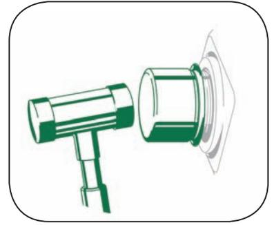
Tap installation tool with mallet until sleeve is seated on shaft over the marked area. Remove installation tool.\*
