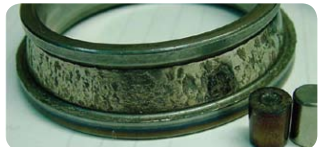
Raceway spalling occurred after 10 minutes of a 6 hour test.
