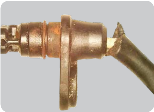
Improper sensor head overmolding design results in sensor wire breakage.
