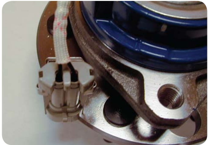
Value grade hub sensor wire diameter is 1.36 mm with an inferior fabric protection sleeve, exposing the sensor to damage from outside elements, wear and heat.
