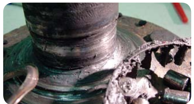
Bearing failure caused by improper press fit between inner ring and hub.
