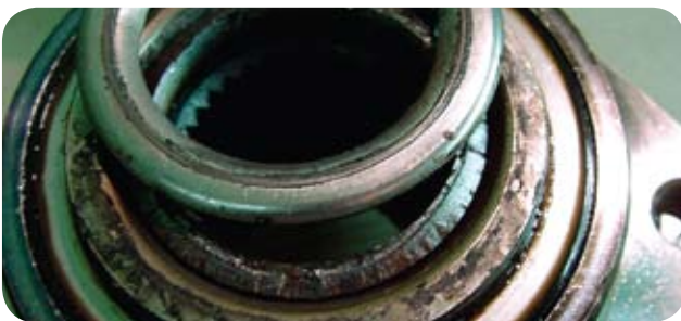
Hub fracture due to flawed roll form design and heat treating process.
