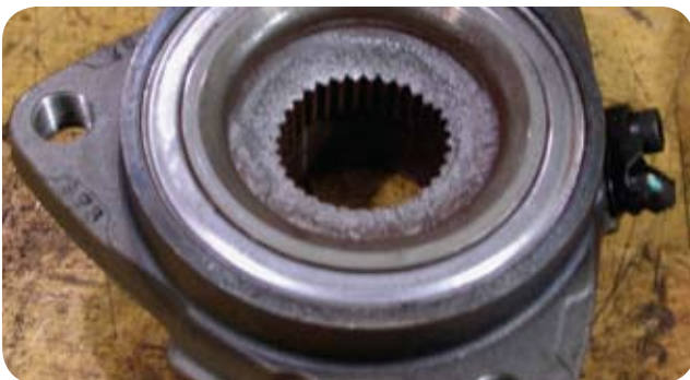
Hub separation caused by poor material specification and improper bearing clearance range.
