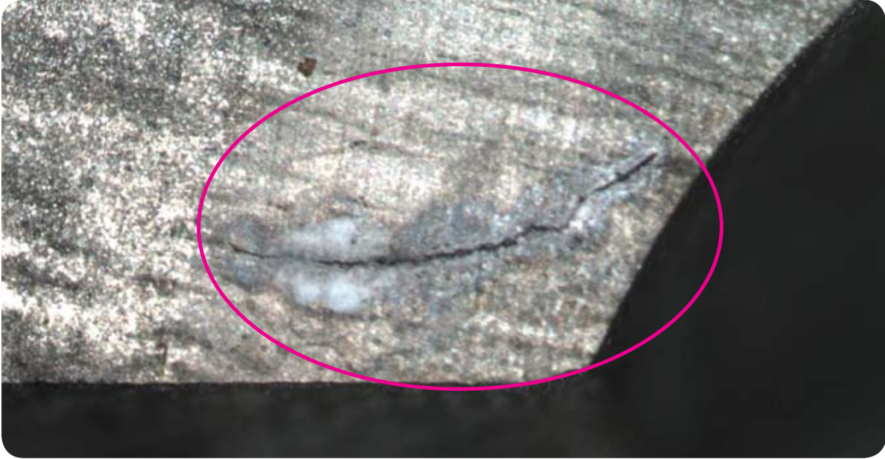
Sub-surface forging crack in the bearing raceway, which will lead to early spalling and eventual failure.
