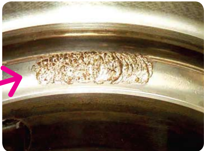
The result was bearing raceway spalling at just 1,000 miles, causing noise and vibration, which would have led to a hub failure soon afterwards.
