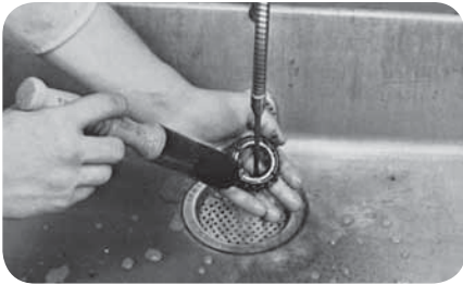
Rinse bearing in clean solvent (fig. 5).
