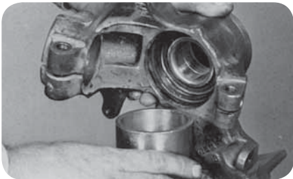
Ford – Place knuckle assembly over spacer tool (fig. 33).
