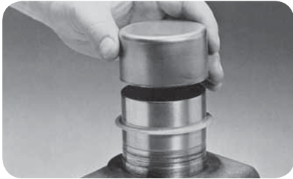
Place Installation tool over Speedi-Sleeve (fig. 46).
