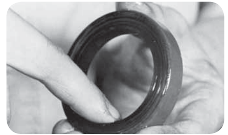
Apply lube to seal lips (fig. 43).
