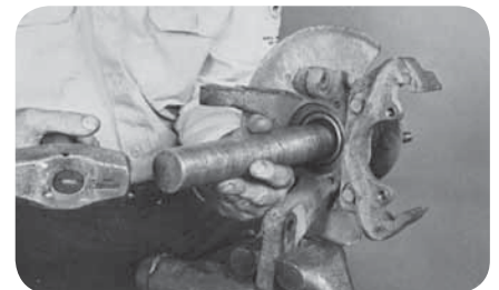
Chrysler – Remove hub from knuckle (fig. 29).
