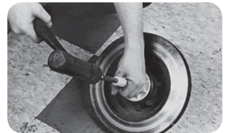
Tap tool until seal is seated in hub (fig. 10).
