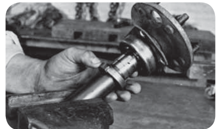
Slide off retainer (fig. 18).
