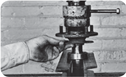
Use arbor press to install bearing (fig. 22).
