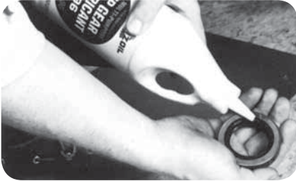
Pre-lube seal with differential lubricant (fig. 19).
