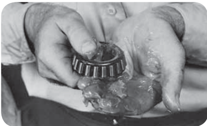
Grease bearing (fig. 7).
