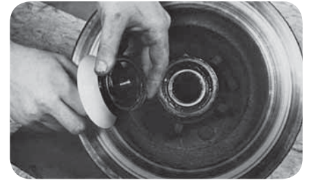
Slide SKF seal onto installation tool (fig. 9).
