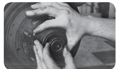
Install outer bearing (fig. 12).
