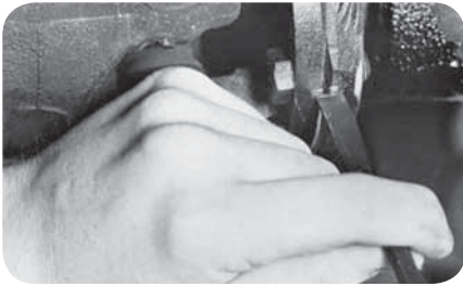
Mark the driveshaft and pinion flange (fig. 39).
