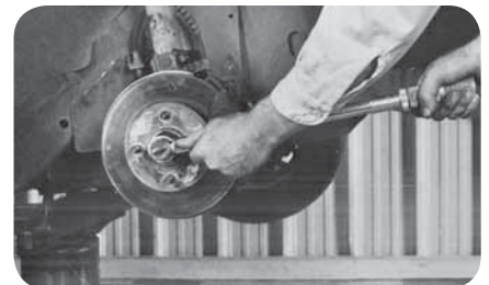
Tighten hub nut while applying brakes (fig. 38).
