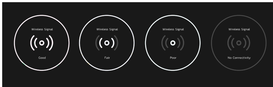
Figure 25. Wireless Extender Signal Strength Indicators
