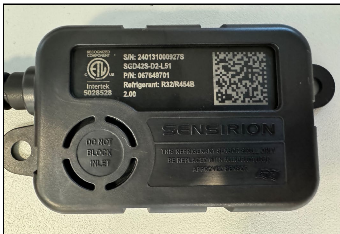
FIGURE 20. Example of Clear, Unobstructed Sensor Inlet
