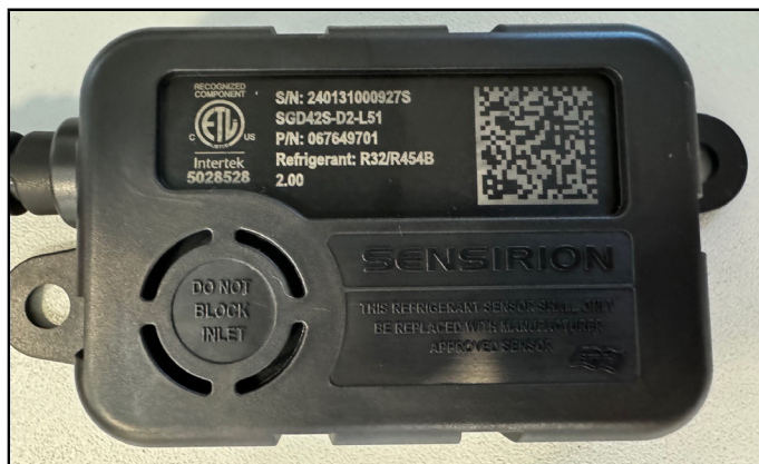
FIGURE 22. Example of Clear, Unobstructed Sensor Inlet
