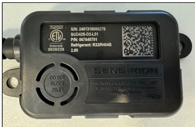
FIGURE 22. Example of Clear, Unobstructed Sensor Inlet
