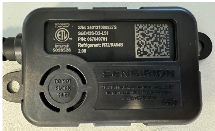
FIGURE 14. Example of Clear, Unobstructed Sensor Inlet
