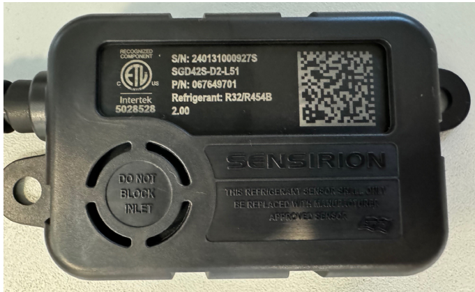
FIGURE 12. Example of Clear, Unobstructed Sensor Inlet
