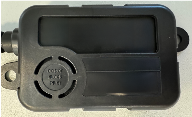
FIGURE 10. Example of Clear, Unobstructed Sensor Inlet
