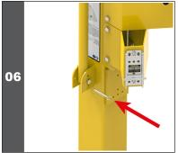
Replace the pin in the handling arm.
