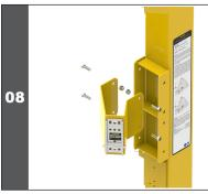
Verify that the self-retracting lifeline and winch bracket (A5039-39) are installed. If necessary, install the bracket on the mast system/davit (IN-5039) using the four (4) nuts and bolts provided with the bracket (A5039-39).
