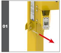
To orient the mast system/davit (IN-5039) in the desired direction, start by removing the pin from the handling arm.
