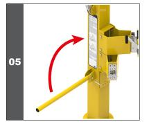
Raise the handling arm when the desired direction of the mast system/davit (IN-5039) has been reached.
