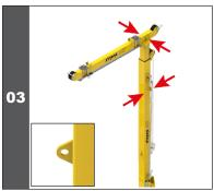
With the help of the available lifting equipment, lift the mast system/davit (IN-5039) using the two (2) lifting points on the mast system/davit (IN-5039).
