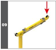
Insert and thread the cable of the self-retracting lifeline or winch cable as far as the second pulley, situated on the front edge of the mast system/davit (IN-5039).
