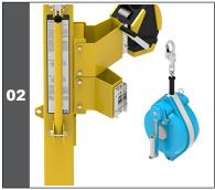
Install the self-retracting lifeline or winch onto the bottom bracket (A5039-27). Verify that the compatible mounting plates are used for the installation. Use the locking pin, provided with the bracket (A5039-27), to lock the self-retracting lifeline or winch.
