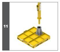
Insert the mast system/davit (IN-5039) into the floor adapter (IN-5040).
