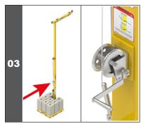
Adjust the height of the mast system/davit (IN-5039) using the crank.
