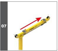
Thread the cable of the self-retracting lifeline or winch cable as far as the second pulley, situated on the front edge of the mast/ davit.
