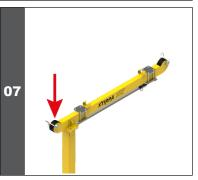
Insert and thread the cable of the self-retracting lifeline or winch cable as far as the first pulley, situated on the back edge of the mast system/davit (IN-5039).
