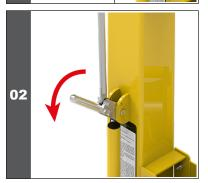
Lower the handle on the locking mechanism to unlock.
