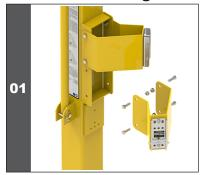
Install the bottom bracket (A5039-27) on the mast system/davit using the four (4) nuts and bolts provided with the bracket (A5039-27).
