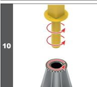
Before inserting the mast system/davit (IN-5039), apply approximately 16 oz (454 ml) of all-purpose grease -0.4 °F to 257 °F (-18 °C to 125 °C) around the base of the mast system/davit (IN-5039) and approximately 2 oz (57 ml) on the interior surface of the floor adapter (IN-5040).
