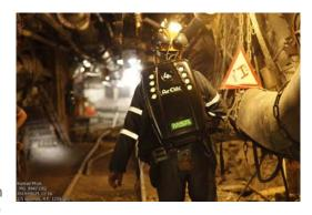
The training set offers a capacity of 120 minutes at a breathing rate of 40 l/min., providing the user with the same high quality of air as the real device. It has been proven that the user will be most comfortable with oxygen comsumption greater than 80% and low humidity between 20% and 40%, thereby limiting the physical exertion required. The set weighs less than 15 kg and has excellent ergonomics with most of the weight borne by the hips.
