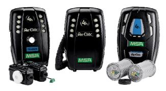
With technical values such as -1.5 mbar inhalation and +3 mbar exhalation resistance at 30 l/min with Advantage filters, the AirElite provides the same amount of resistance for training as when using the real 4-hour canisters.
