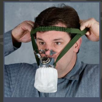
Take off headgear and pull harness over head. Put lower strap behind the head, and upper band above the forehead as shown. The head harness will support the weight of the respirator.
