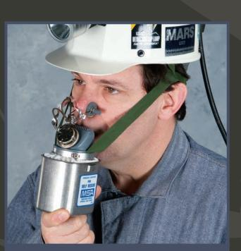
Before going underground, every miner should examine his Self-Rescuer for any external damage. If the container is dented, it may not be possible to remove the respirator from the container. In this case, the wearer can still breathe with the filter and the inner wall in the container. The space between the filter and the inner wall is large enough to allow normal breathing. Because of the greater weight, it would be advisable to ease the load on the teeth and jaw by
