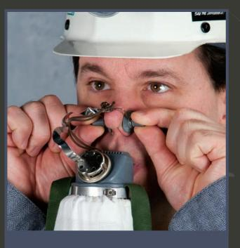
Pull the pads of the noseclip apart and position pads over the nostrils.
