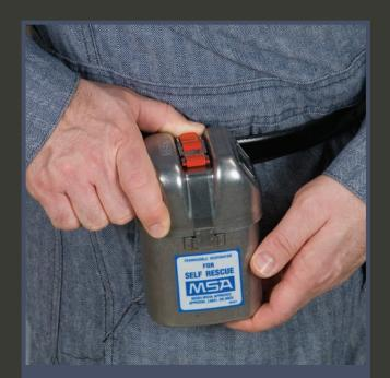
Release the locking device by pressing the thumb under the red release lever and pushing up ...
