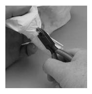
2. Pull the hood tube and suspension out of the hood.
