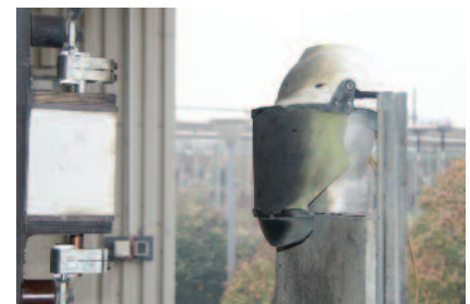
GS-ET-29 class 2-7 kA certification passed. Head and face combination protects the wearer
