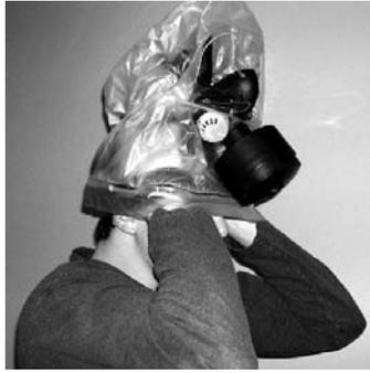
8. Ensure the neckseal is sealed against neck. Nothing should be obstructing the neckseal to the skin.
