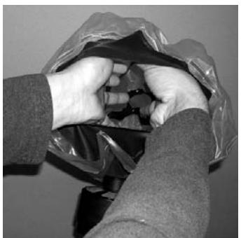
3. Adjust the nosecup on the face until it is comfortably covering both the nose and mouth.
