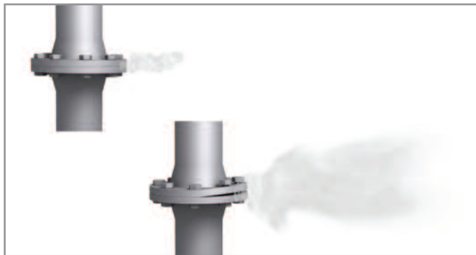
Figure 8. When the pressure is kept constant a small leak has a smaller leak rate and makes less ultrasound compared to a bigger leak.
