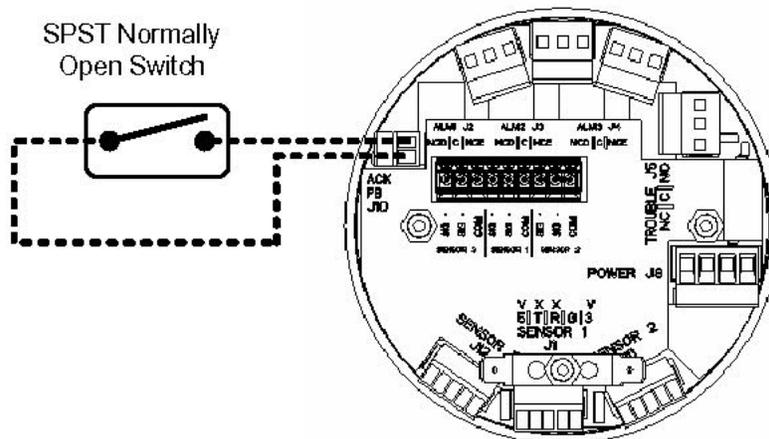
**Figure 2-4. Push-button Wiring**
