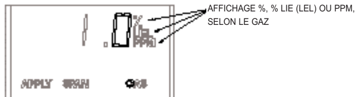
Figure 2-6. Message Apply SPAN Gas
