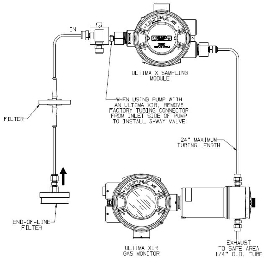
**Figure 1-2. Sampling Module Installation with Ultima XIR Sensors**
