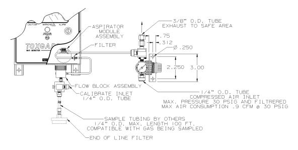
Fig. 37 Typical Air Aspirator Version Installation
