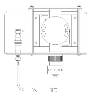
Fig. 45 Ultima Duct Mount Kit
