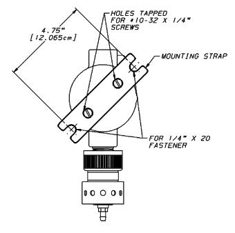
Fig. 5 Remote Sensor Mounting Method
