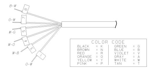
Fig. 12 Toxic Gas Remote Sensor Cable
