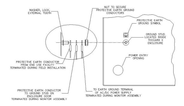
Fig. 7 Connection of Protective Earth Ground Conductors
