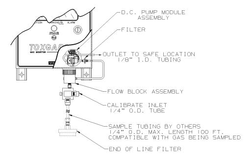
Fig. 36 Typical DC Pump Version Installation
