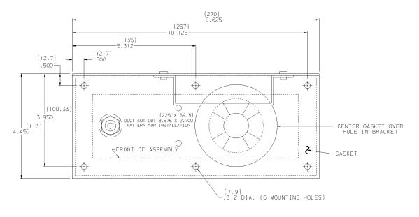
Fig. 46 Duct Template
