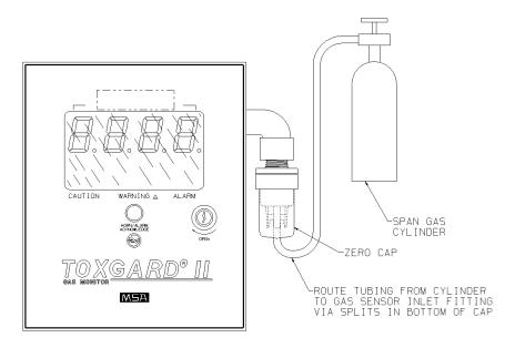
Fig. 31 Zero Gas Connection
