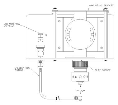
Fig. 51 Duct Mount and Sensor
