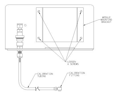
Fig. 50 Remote Sensor Base Plate
