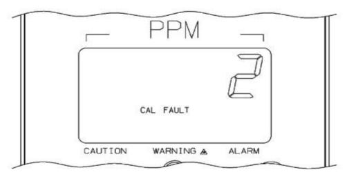
Fig. 44 CAL FAULT Reading
