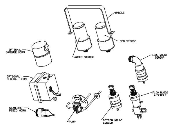
Fig. 4 Options and Accessories (Battery Back-up not shown)
