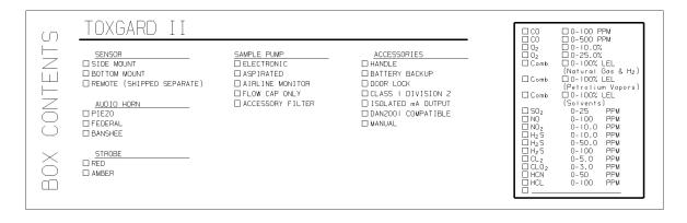
Fig. 3 Shipping Carton Label Identifying Sensor Type
