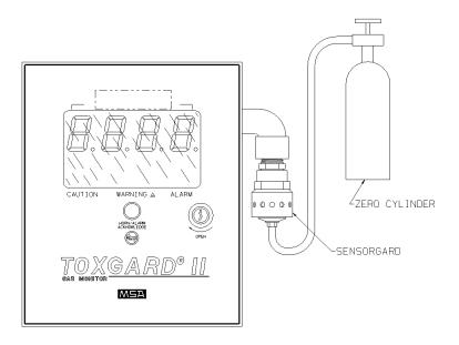
Fig. 26 Zero Gas Connection
