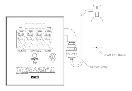
Fig. 33 Span Set-up
