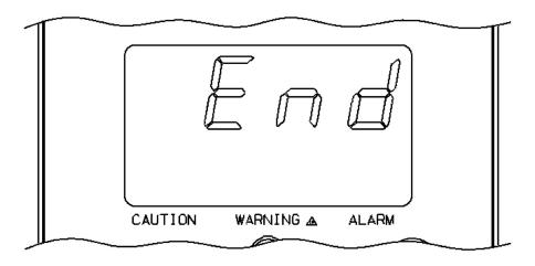
Fig. 34 Calibration End Display
