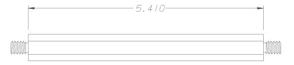
Fig. 47 Remote Sensor Spacers
