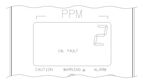
Fig. 29 Calibration Fault Flag
