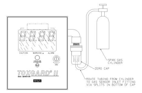
Fig. 35 Span Gas Connection
