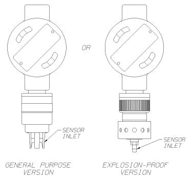
Fig. 2 Remote Sensor Model
