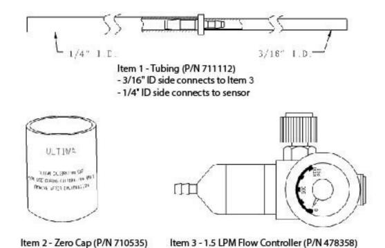
Fig. 19 Calibration Kit 40 Contents (Your Kit may also include one or two gas cylinders)
