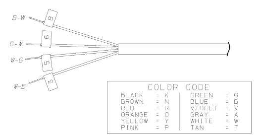
Fig. 10 Oxygen Remote Sensor Cable
