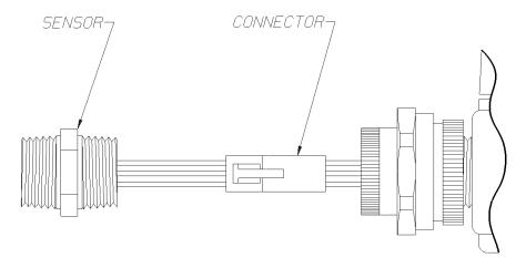
Fig. 43 Combustible Three-Pin Connector
