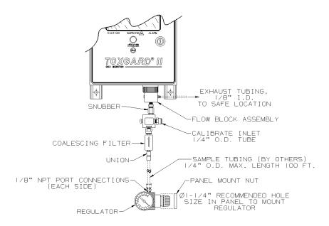
Fig. 38 Typical Air Line Monitor Installation
