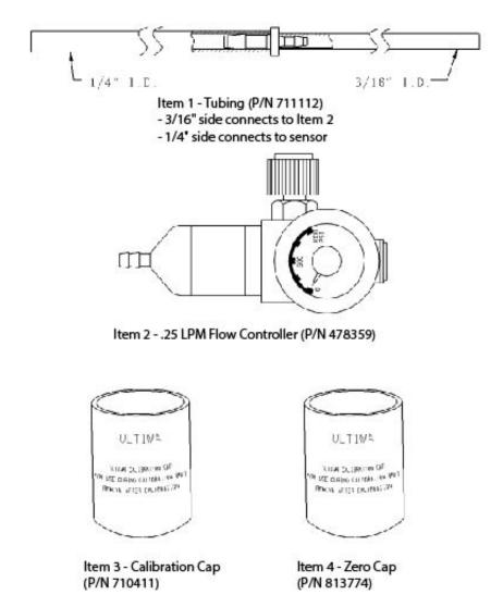
Fig. 20 Calibration Kit 41 Contents (Your Kit may also include one or two gas cylinders)
