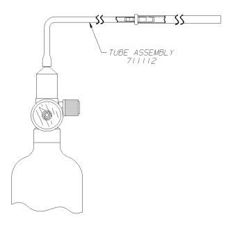
Fig. 25 Calibration Tubing Set-up
