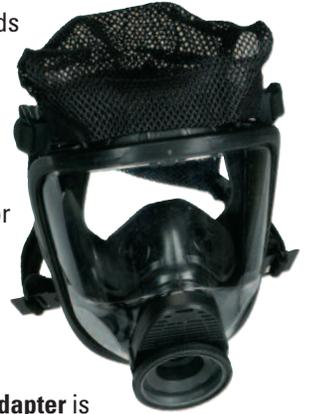
MSA's **Push-To-Connect (P-T-C) Adapter** is approved with the AirHawk SCBA and installs easily without special tools. This adapter provides both inhalation check valve and exhalation valves, preventing exhaled air from entering and contaminating the mask-mounted regulator.
