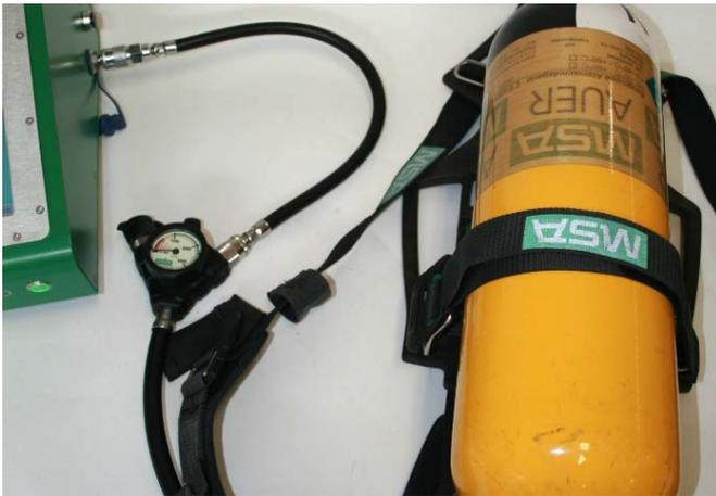
Fig. 35 Connecting Breathing Apparatus
