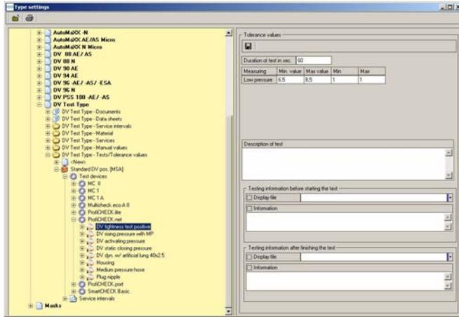
Fig. 107 Menu: Technical Services – Settings – Check tolerance values
