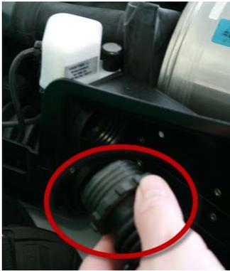
Fig. 46 Screwing adapter into exhalation side
