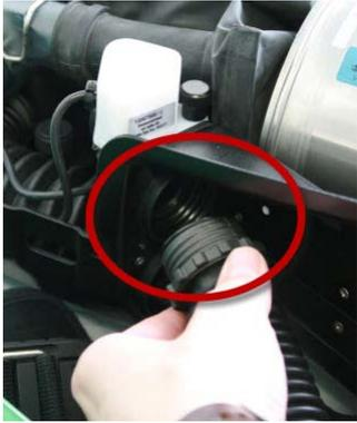
Fig. 45 Screwing adapter into inhalation side
