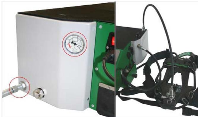
Fig. 36 Connecting high pressure line
