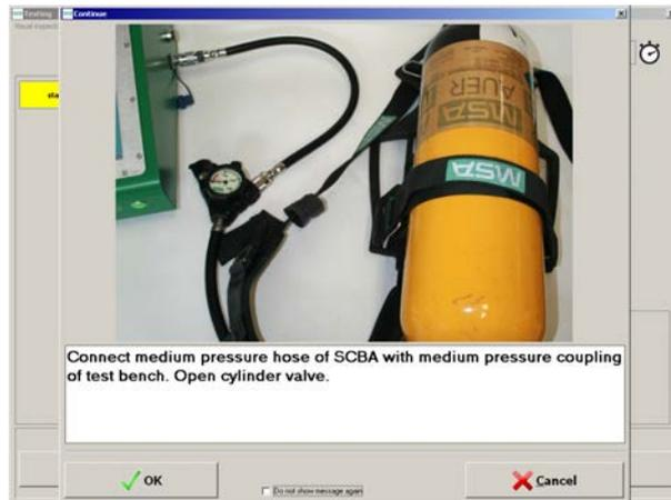
Fig. 37 Connecting the compressed air breathing apparatus
