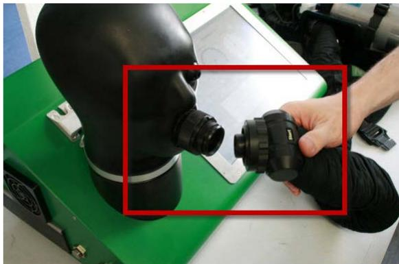
Fig. 47 Connecting breathing hose assembly to test head
