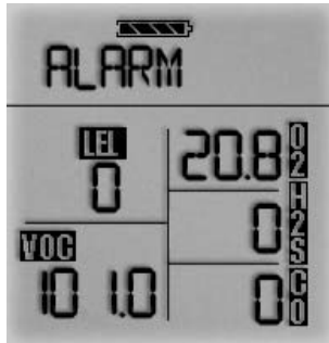
Figure 3-7b. Instrument in VOC Gas Alarm
