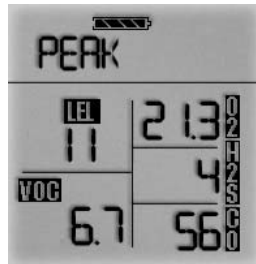
Figure 3-10. PEAK Readings on the Display
