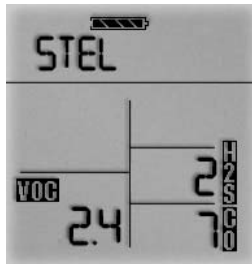
Figure 3-12. Exposure Page with STEL Alarm
