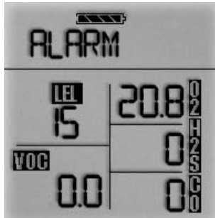
Figure 3-5b. Instrument in LEL Alarm
