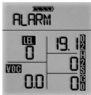
Figure 3-6b. Instrument in Oxygen Alarm
