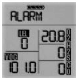
Figure 3-7b. Instrument en alarme COV
