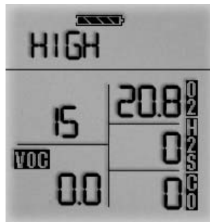
Figure 3-5a. Instrument in LEL Alarm
