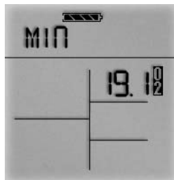
Figure 3-11. MIN Reading on the Display
