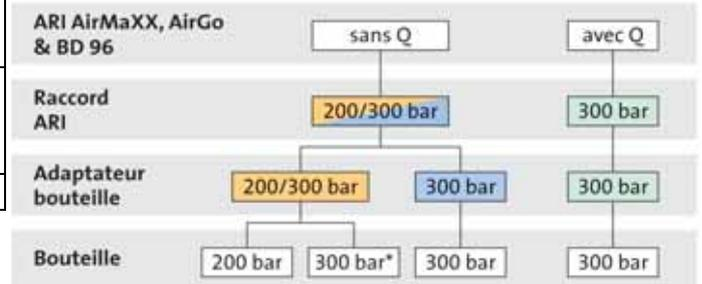
Q = Connexion QuickFill
