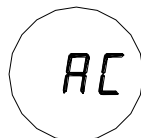
Figure 21: Automatic Calibration Mode
