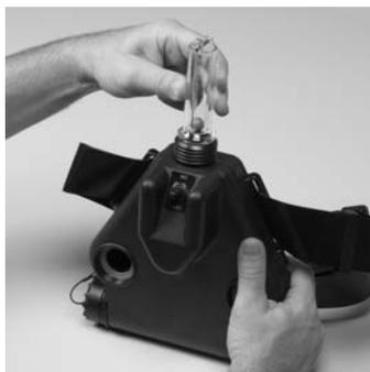
4. Position the blower assembly in an upright position so the airflow indicator is vertical on top of the blower assembly.
