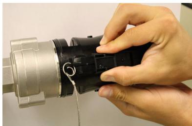
Fig. 18 Remove Environmental Guard
