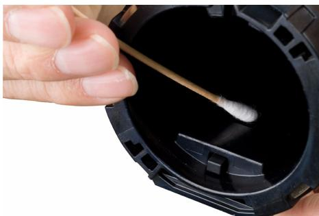
Fig. 21 Calibration cap diode cleaning
