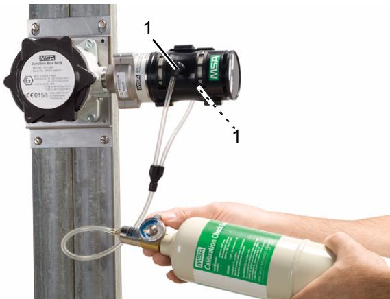
Fig. 15    Remote HART calibration set-up
