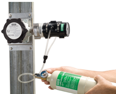
Fig. 11 Bump Check setup with environmental guard
