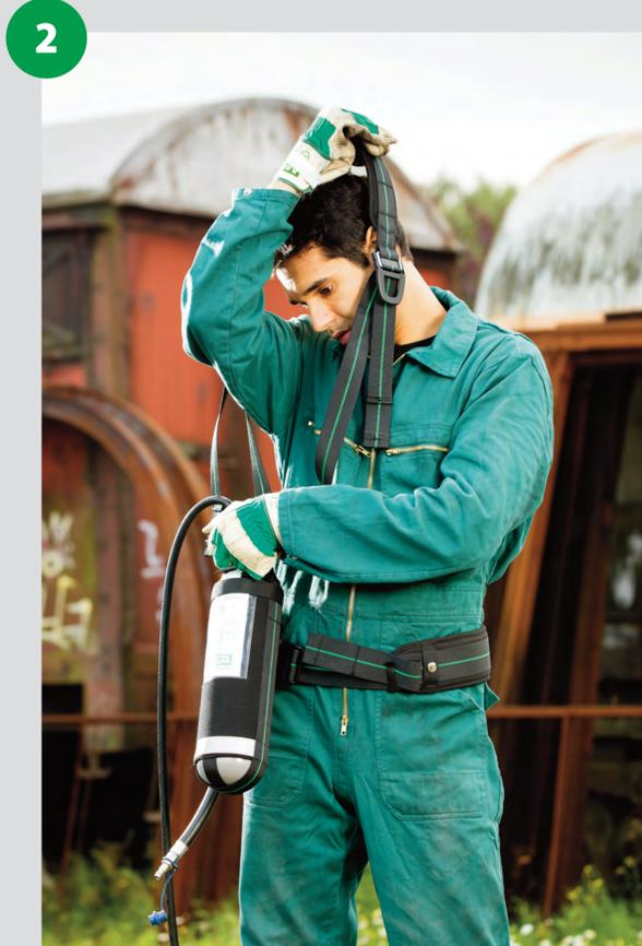
2 Put on shoulder harness with cylinder demand valve airline assembly.
