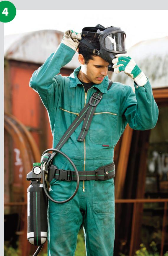
4 Put on facepiece, adjust harness straps and test facepiece tightness.
