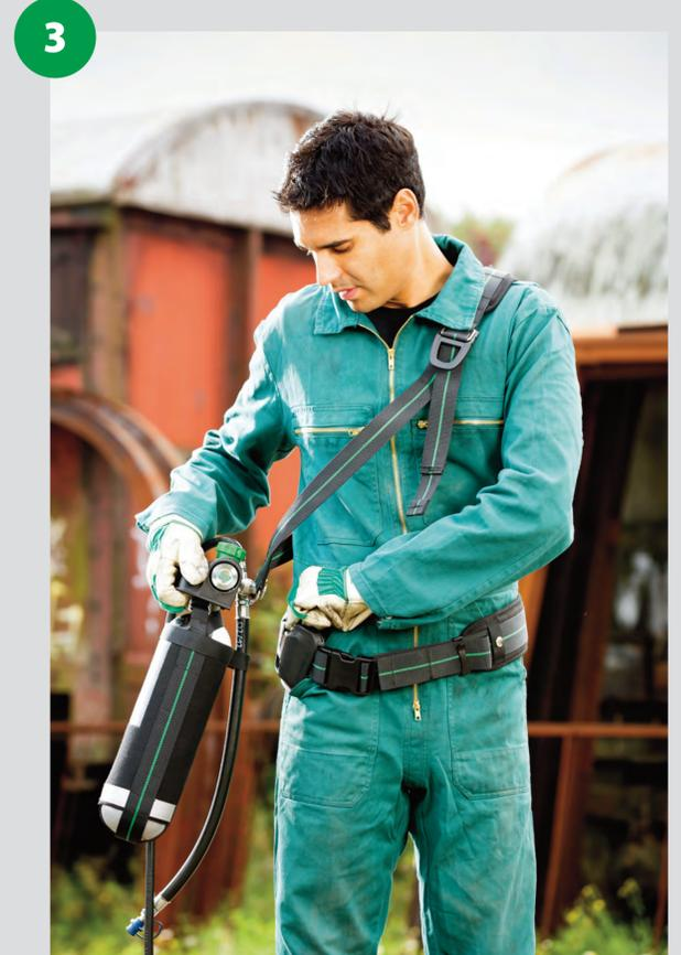
3 Attach cylinder to holster assembly and adjust shoulder strap.
