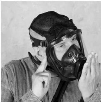
**NOTE:** It may be necessary to exhale sharply to open the valve. If this does not release the valve, do not use the facepiece.
