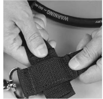
9. Connect the pull strap to the cylinder carrier D-ring to the right of the pressure gauge (when looking at the gauge).
