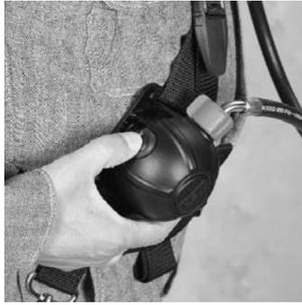
3. While pressing the release buttons, pull the regulator out of the stand-by mount.
