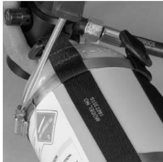
5. Rotate the straps 180°. The straps should be equally spaced on either side of the pressure gauge.
