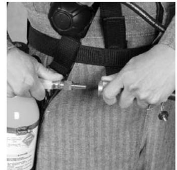
5. Open the bypass to vent system pressure. Close the bypass.
