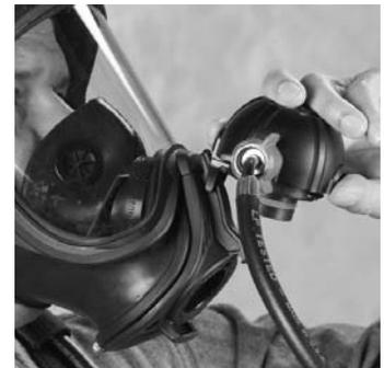
4. Disconnect the attachment hose from the air supply hose.
