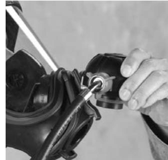
2. Slide regulator onto rail (fast track) of facepiece cover. Slide regulator down the rail cover until regulator stops.
