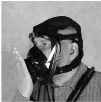
**If it does not, adjust the facepiece and test again. If adjustment does not provide a proper seal, do not use the facepiece.**
