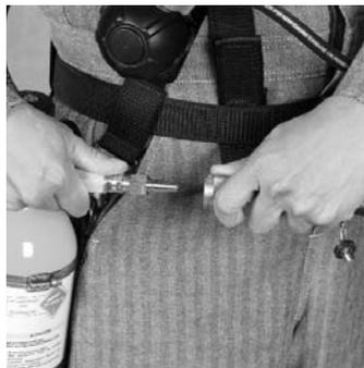
4. Open the bypass to vent system pressure. Close the bypass.
