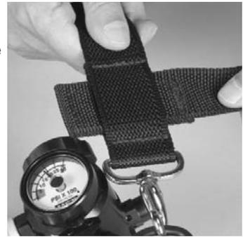
8. Connect the shoulder strap to the remaining cylinder carrier D-ring.
