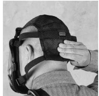
4. Tighten the lower straps first by pulling them straight back, not out. Tighten the facepiece until the mask is snug against the face.
