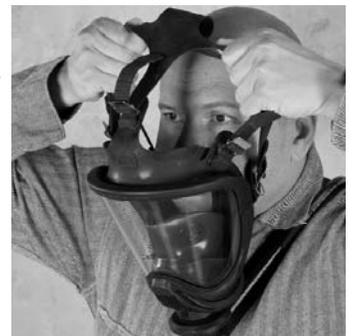
3. Tighten the lower straps first by pulling them straight back, not out.
