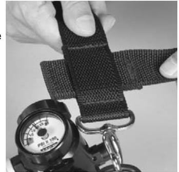
10. Connect the shoulder strap to the remaining cylinder carrier D-ring.
