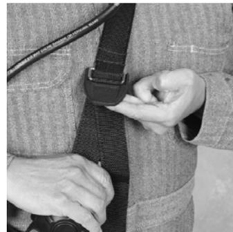
3. Slide the carrier and harness up and over the head.
