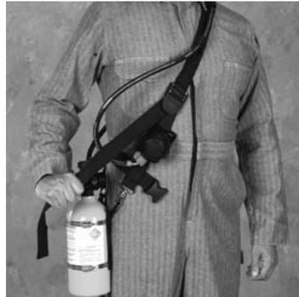
**NOTE:** The cylinder should be positioned at or just below waist level.
