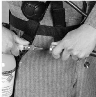
5. Pull on the quick-disconnect plug and socket to verify that the hoses are securely attached.
