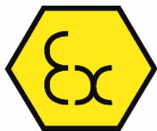
ATmosphere EXplosible is French for potentially explosive atmospheres. According to ATEX manufacturer directive 94/9/EC (ATEX 95) and user directive 1999/92/EC (ATEX 137) the electrical safety of all electronic gas detectors and personal monitors used in potentially explosive atmospheres must be tested and marked "ATEX" (EN 60079-0 et seq.).
