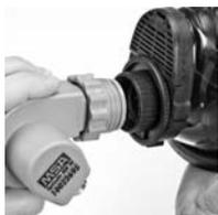
4. Check that there is a gasket in the motor-blower housing. The gasket is necessary so that the filter and motor-blower will seal.
