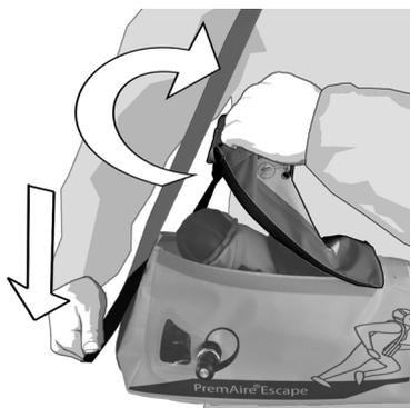
If the bag cannot be opened as described above (e.g. while standing on a ladder), open the velcro fastener first partially on one side with two fingers. Then open the bag completely by pulling on the yellow loop to activate air supply.
