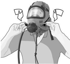
(2) Loosen the head straps: Press the buckles forwards to open the harness.
