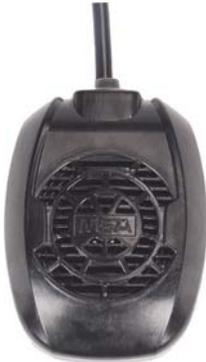
The speaker module amplifies and clarifies the speech from the facepiece during use. When inhaling, the breathing sound will not be amplified (optional). The speaker module is turned OFF when the complete SCBA is turned OFF and can also be activated/deactivated with its button. Pressing of the button is acknowledged by a beep.
