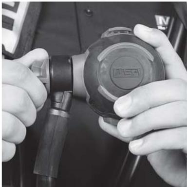
Check the regulator's bypass operation.
