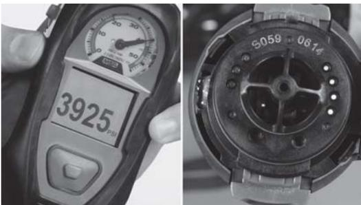
(11) As the system pressure rises from 0 to 200 psi, both visible and audible alerts activate automatically, indicating that the SCBA is functioning properly. The following indications must occur:
