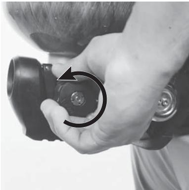
(10) Reach behind and fully open the cylinder valve.
