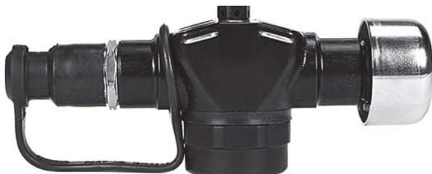
The pressure reducer reduces the cylinder pressure to an intermediate pressure, which is in turn further reduced by the regulator to a pressure that is respirable by the user. The pressure reducer incorporates a fail safe design which ensures air flow to the user in the event of a malfunction within the pressure reducer.
