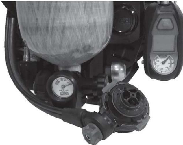
When testing the control module, check if the graphical display and the analog gauge are consistent within 5% of the full cylinder pressure (110 psig for 2216 psig system, 225 psig for 4500 psig system, 275 psig for 5500 psig system).
