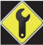
The G1 SCBA can be configured so that an overhaul alarm will appear on the control module after 600 hours of on air usage have elapsed. The overhaul alarm will appear on the control module during startup every time the SCBA is turned on until the overhaul alarm is reset. For detailed instructions on how to turn on the overhaul alarm, refer to the **A2® Accountability Control Software Operating Manual, 10162374**.
