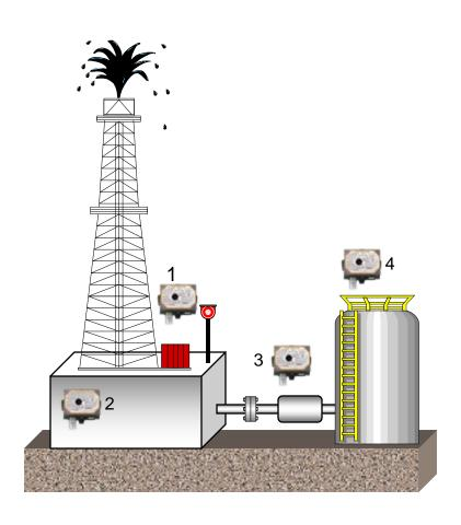
Leaks, such as blowouts in oil drilling applications, quickly release large quantities of H<sub>2</sub>S gas into areas around the drilling site. Model S4000TH Intelligent Sensors are used for this application because of their ability to respond to large concentrations of H<sub>2</sub>S for short periods.
