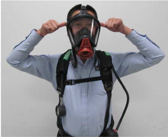
Fig. 20 Loosen stainless steel buckles
