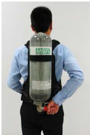
Fig. 13 Open cylinder valve
