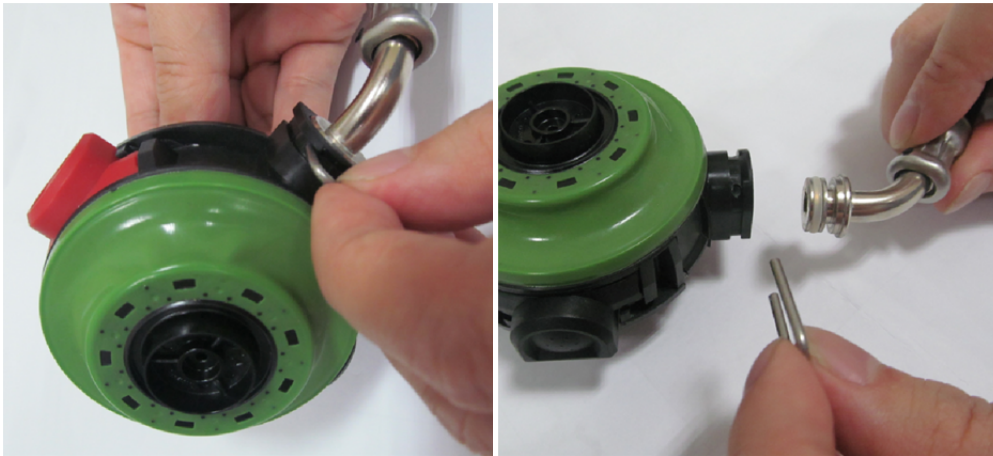
Fig. 25 Disassembly medium pressure line
