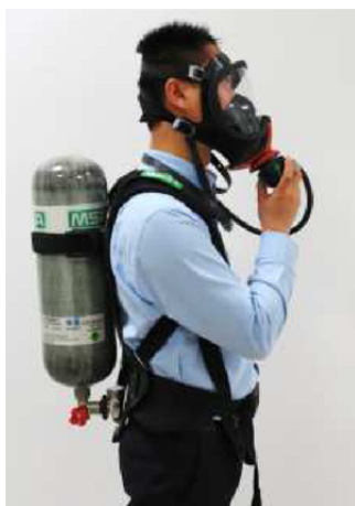
Fig. 18 Connect demand valve with mask
