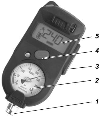
**Fig. 15** *Integrated Control Unit ICU*
