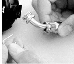
**Fig. 30** *Disassembly medium pressure line*
