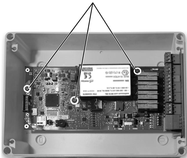
Fig. 6 PCB fixing screws
