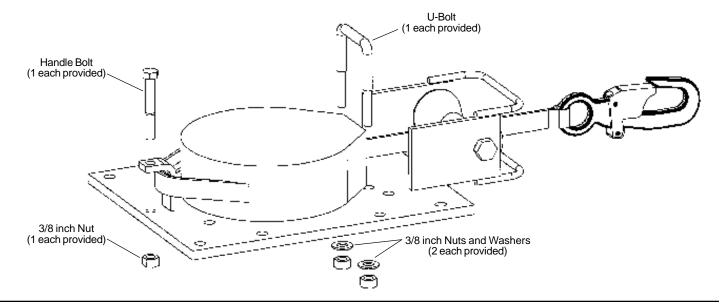
STEP 3 Weave web lifeline between the bracket and roller as shown in the diagram below. Web Lifeline Roller Retractable Lanyard Mounting Bracket
