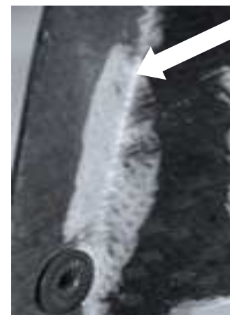
Examples of white marks on the carbon rim of the impact cap.
