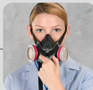
Place facepiece into position and lock down.
