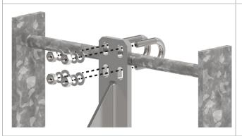
Secure the anchor onto the top ladder rung with the U-bolts and fixings from the top anchor fixing kit. Hand tighten nuts to hold anchor in position.
