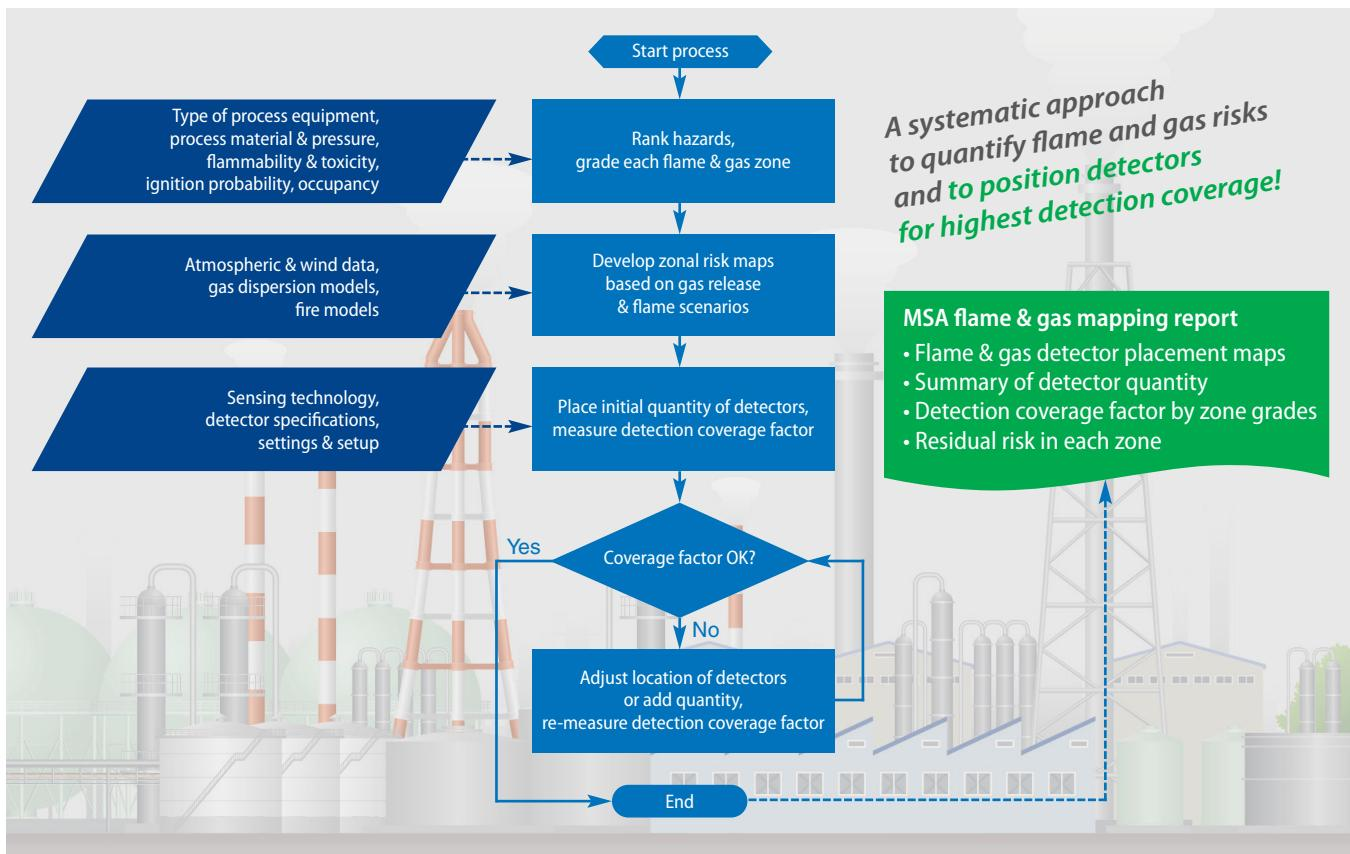
Figure 2 : MSA's flame and gas mapping study approach
